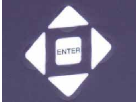
Figure 3-1. Front Panel LCD Display and Five Pushbuttons (Enter, Up, Down, Left and Right)
