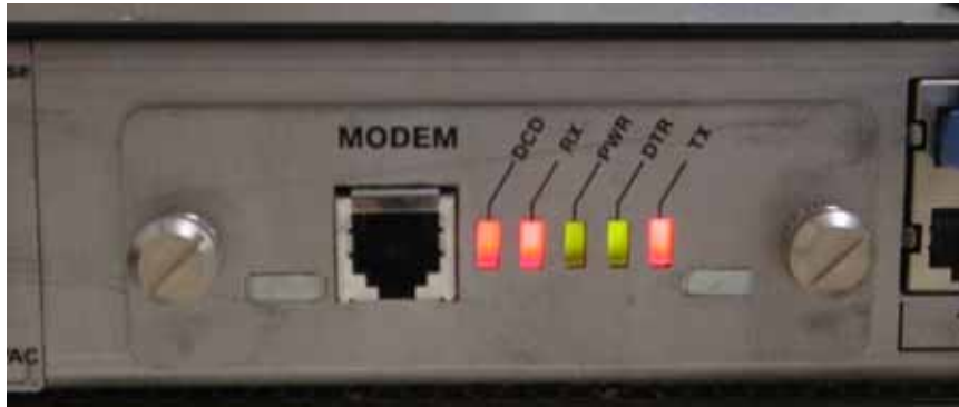
Figure 6-2. Normal Modem LEDs (Red-Red-Green-Green-Red) for an idle Modem Port
