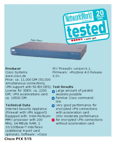
However, running Cisco with the acceleration cards is a whole different scenario. Handling 512 Byte-long packets, PIX reaches 51% throughput in the uni-directional mode and 25% in the bidirectional mode. This means that hardware accelerators provide a 5 times performance improvement when handling 512 Byte-long packets. Due to the high processor capacity, the throughput values of Astaro, based purely on software encryption, are very good.
