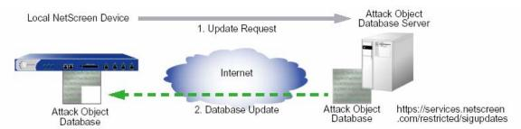
The update process entails connecting to the Juniper Attack Object Database Server, which will be updated regularly with new attacks and updates to preexisting attacks. Emergency updates will also be provided to protect against key attacks as necessary. Customers must have a software subscription and subscribe to the Target Attack Update Service to receive these new attack protection enhancements.
