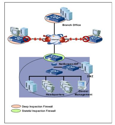
By layering the Juniper integrated firewall/IPSec VPN systems and appliances and IDP solutions throughout the enterprise network, organizations can maximize their security while minimizing their overhead. Obviously the most critical resources must be protected at all costs, so by layering the firewall functionality in this manner increases an organizations ability to mitigate both network and application-layer attack.
